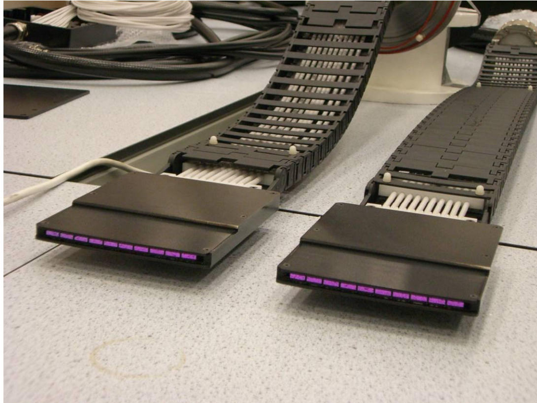
Fibres immersed to glass meniscus with A/R coating
