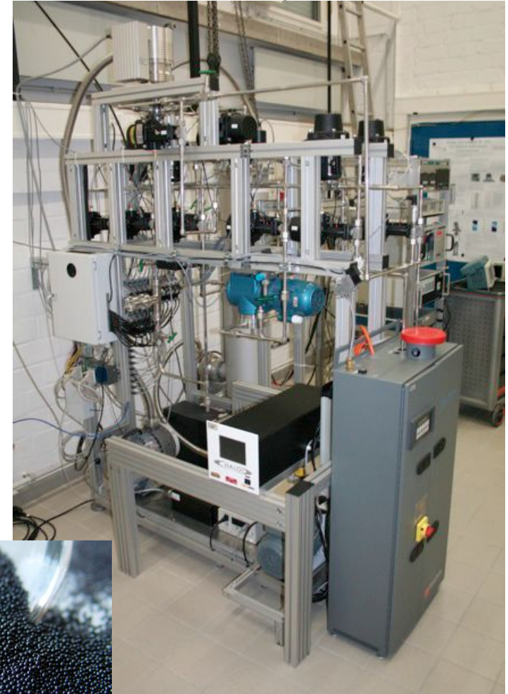
Xe purification system
