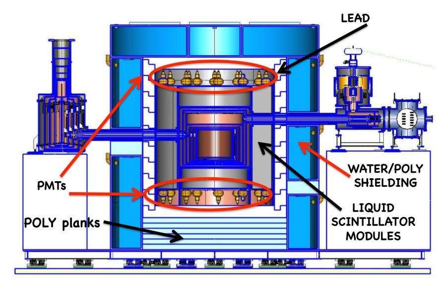
Neutron veto modules filled with Linear Alkylbenzene (LAB), read out by PMTs
