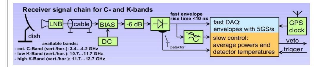
Dish – feeds – LNBs – power supply and detector – scope – gps clock - pc
