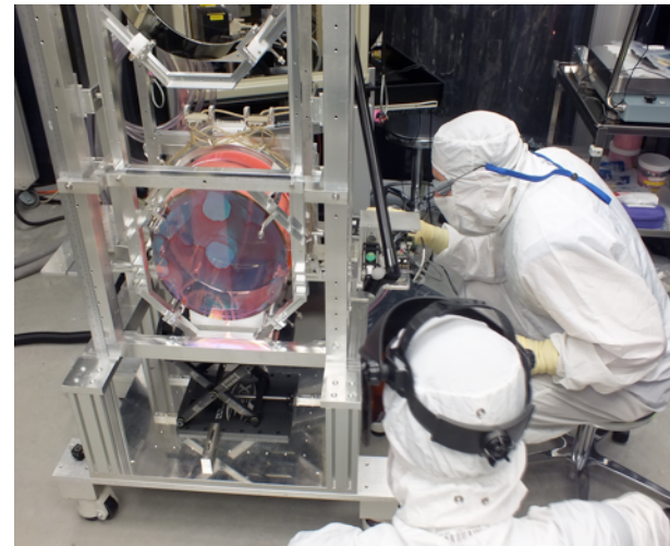
Welding the LIGO Livingston X-arm Input Test Mass to Fused Silica Fibers
